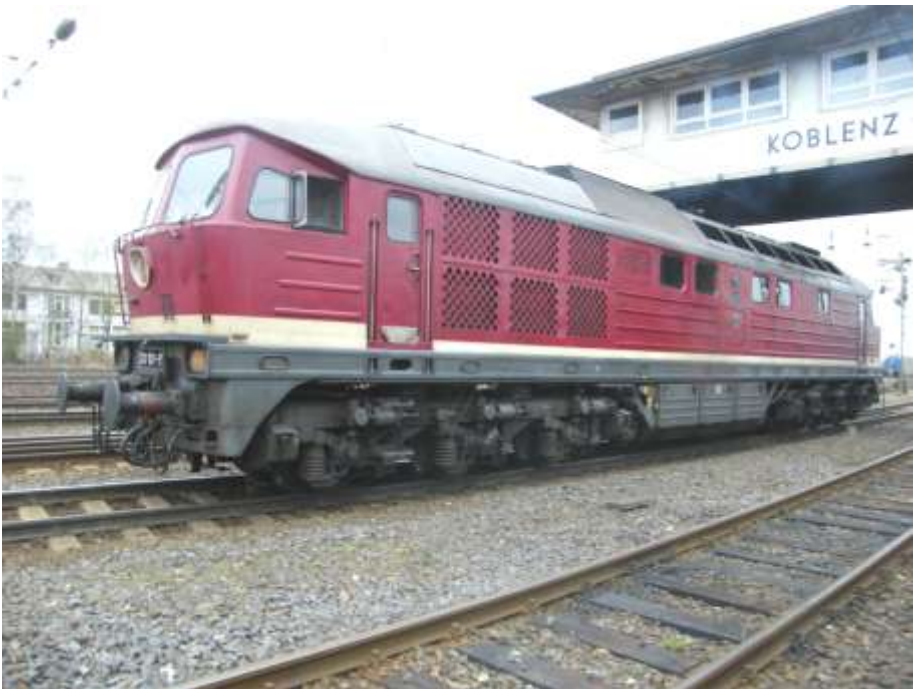
DB 130 101-9 - Voroshilovgrad (now Lugansk, Ukraine)-built Co-Co (Soviet export class TE109) at Koblenz Lutzel depot, (DB175 event) ,11 April 2010 Gary Hayhurst
